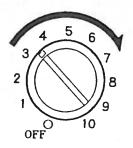
When this dial is turned clockwise from the OFF position a click will be heard and the unit will be switched on. At this time the Soundome will be automatically lowered. Further clockwise turning of the dial will brighten the screen display. When the power is turned off, by turning the dial anti-clockwise, the Soundome will be raised automatically.
